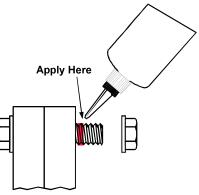
6. **For Blind Holes**, apply several drops down female threads into the bottom of the hole. As threads are engaged, <u>compressed air forces the product upwards into the threads</u>.
